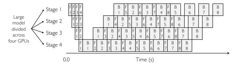
One training iteration with 4 pipeline stages and 8 microbatches (IFIB schedule).
