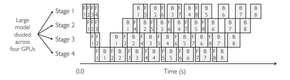
One training iteration with 4 pipeline stages and 8 microbatches (IFIB schedule).
