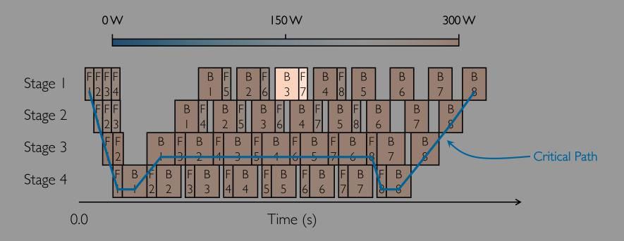
One training iteration with 4 pipeline stages and 8 microbatches (IFIB schedule).
